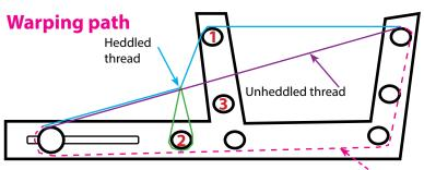
Note how the heddle pulls the warp thread it it controlling into the same plane as the unheddled warp thread that goes from the front peg to the back peg. If the heddle is too long or too short, it will affect the ability to get a good shed.
